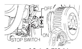
Figure 5. Engine On/Off Switch
